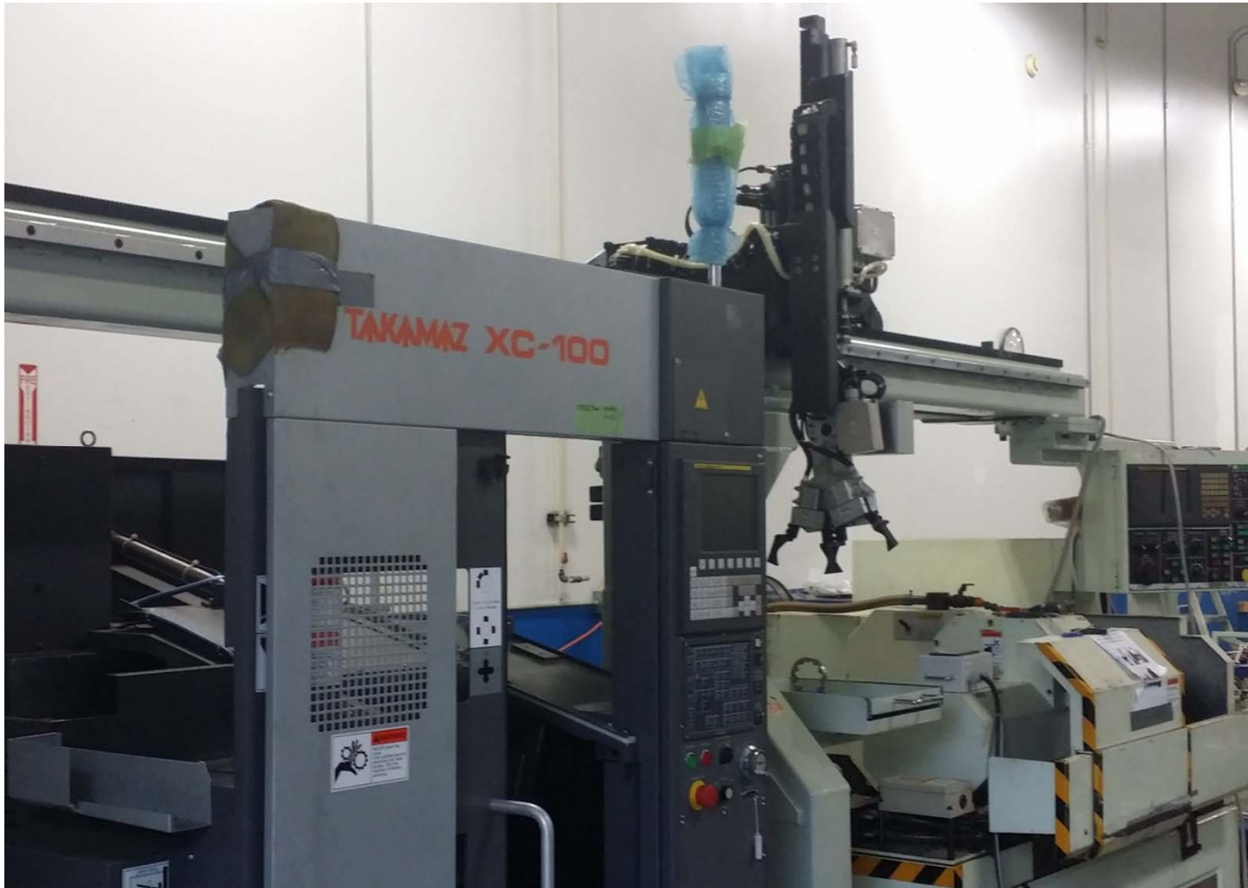
Pump Gear In-process Gantry Loader
